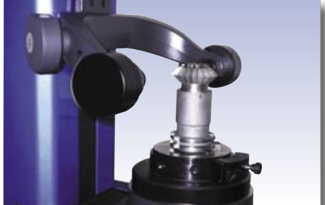
Checking of a champher cutter
