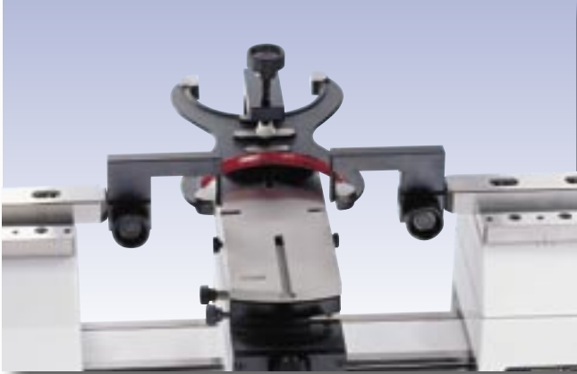
Checking of snap gauges from 12 to 150 mm (LABC-13, TEL14N, TEL16.1)
