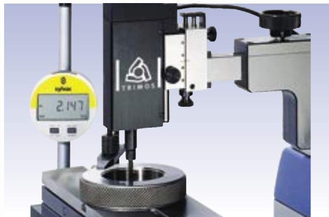
Checking of thread ring gauges (HPA-13, LABC-70, TEL75)
