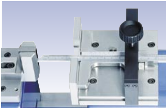
Checking of depth gauges (TEL5, TEL19.1)
