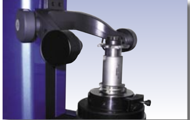
Checking of a side cutter
