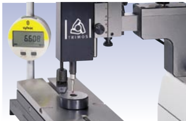
Checking of ring gauges (LABC-13, TEL14.1, TEL14.2, LABC-70, TEL76)
