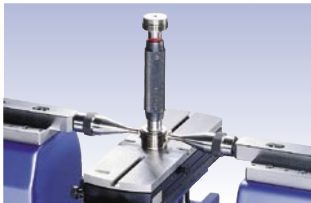
Checking of thread plug gauges (HPA-13, TEL14.1, TEL14.2, TEL6, 3P/0.17-3.2/S6.5)
