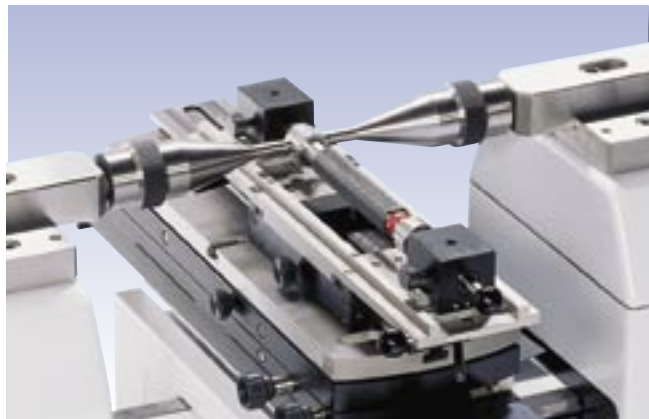
Checking of plug gauges between centers (LABC-13, TELS6, TEL6)
