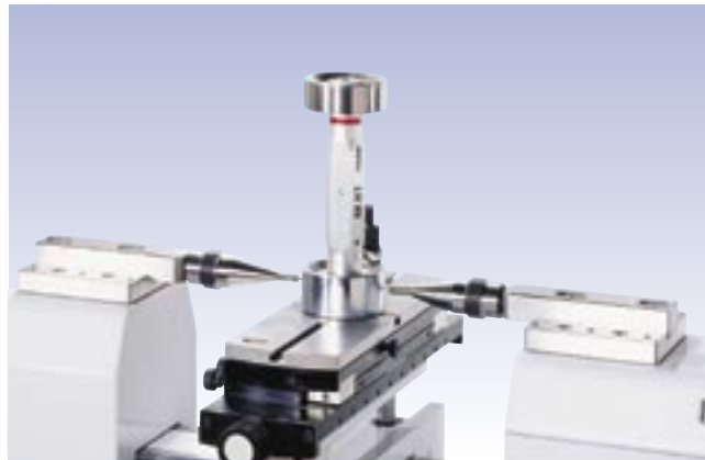
Checking of plug gauges and thread plug gauges (LABC-13, TEL14.1, TEL14.2, TEL6)
