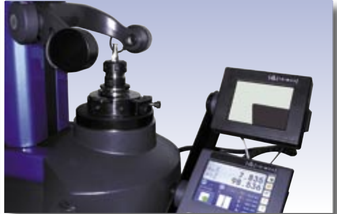
Checking of a two-flute cutter
