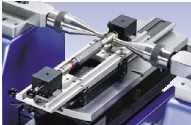
Checking of thread plug gauges between centers (HPA-13, TELS6, TEL6, 3P/0.17-3.2/S6.5)
