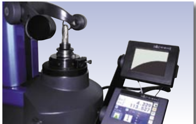
Checking of a radius cutter
