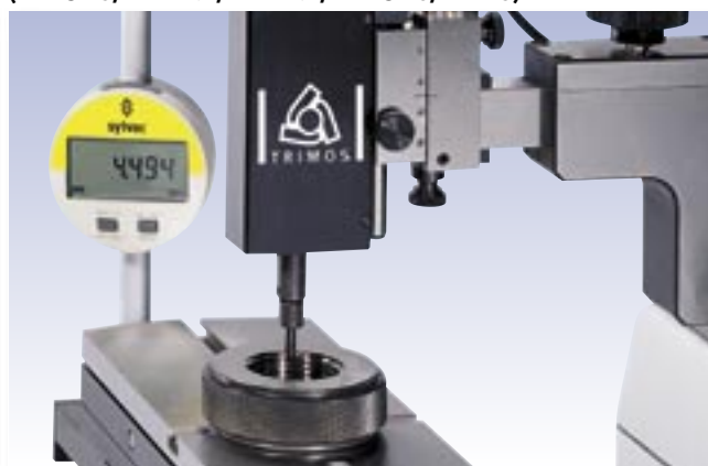
Checking of thread ring gauges (LABC-13, TEL14.1, TEL14.2, LABC-70, TEL75)
