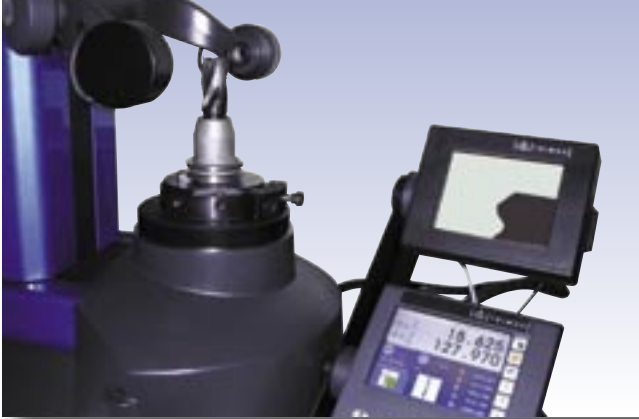
Checking of a thread cutter
