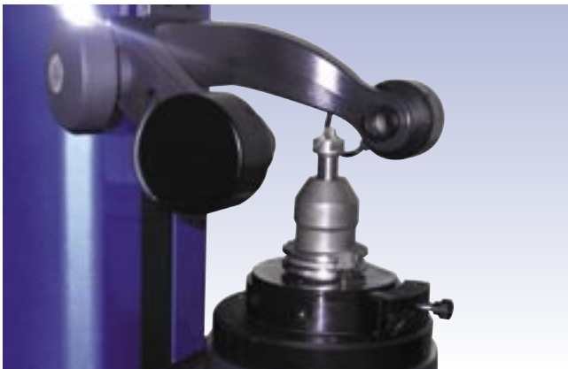
Checking of a quadrant cutter
