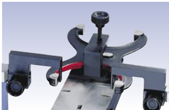
Checking of snap gauges (HPA-13, TEL14N, TEL16.1)
