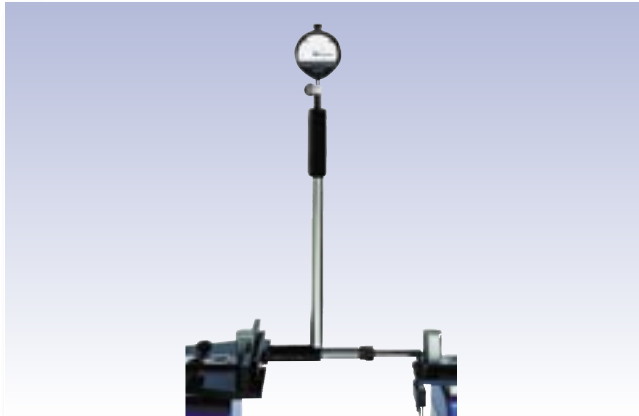
Setting of 2-point bore gauges (TEL5, TEL17.2, TELMN4)
