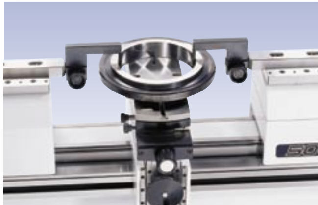
Checking of ring gauges (LABC-13, TEL14.1, TEL14.2, TEL16.1, TEL16.2)
